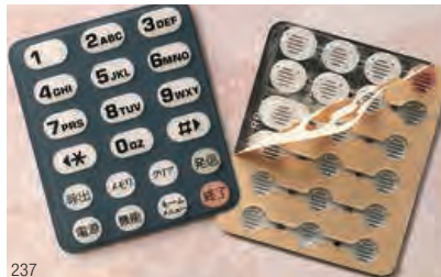
237 With differential adhesive, the silicone adhesive side of 3M™ Double Coated Tape adheres to a silicone rubber keypad. Acrylic adhesive side adheres to a plastic base.
